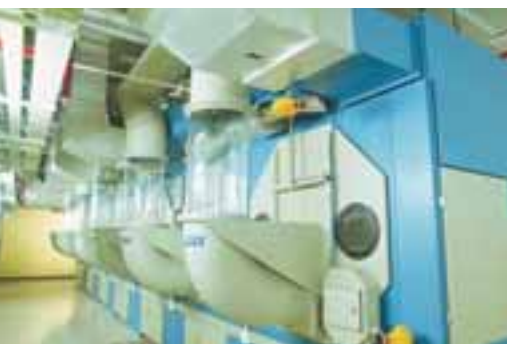
New China Laundry has introduced vacuum transfer system to shorten the drying time and reduce hot air dissipation
